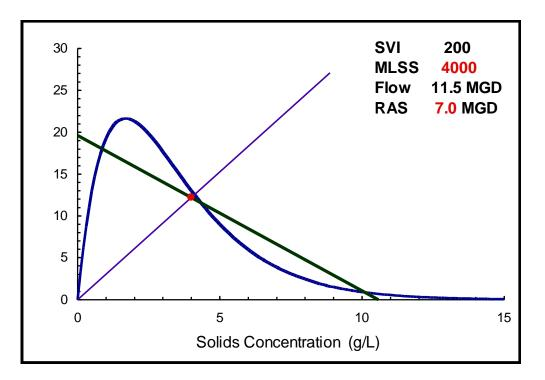
Clarifier #5 State Point Analysis Overloaded, Clarification Failure
