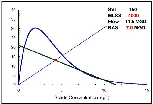
Clarifier #5 State Point Analysis Overloaded, Thickening Failure
