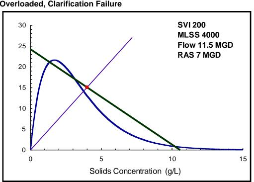
Clarifier #1 State Point Analysis Overloaded, Clarification Failure
